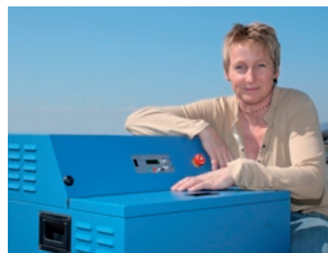
Portable pressure electrolyser with drying unit for filling metal hydride storage
