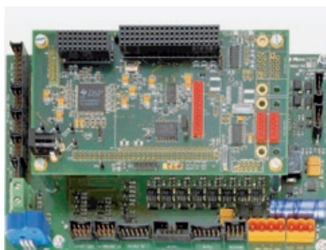
Control electronics for a complete autonomous electrolysis system.
