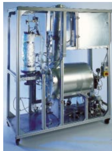
View of entire system for autothermal reforming of diesel. The reactor is in the left upper part of the system.
