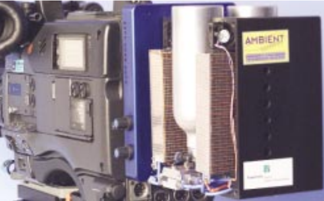
Prototype of a fuel cell system, developed at Fraunhofer ISE, for use with professional film and television cameras. The system has twice the volumetric energy density as compared to a Li-ion secondary battery of similar size.
