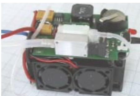
Packaging of a miniature fuel cell system with a power of 10 W including the system components.
