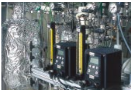
Kerosene reformer for a solid oxide fuel cell (SOFC) with a power of 25 kW and integrated de-sulphurisation.
