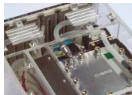
Direct methanol fuel cell system with 30 W steady state power. The system operates with pure methanol.
