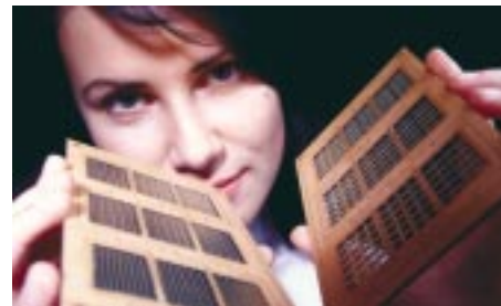
Planar fuel cells with a peak power of 8 W. The series connection of three fuel cells is realised in printed circuit board technology.
