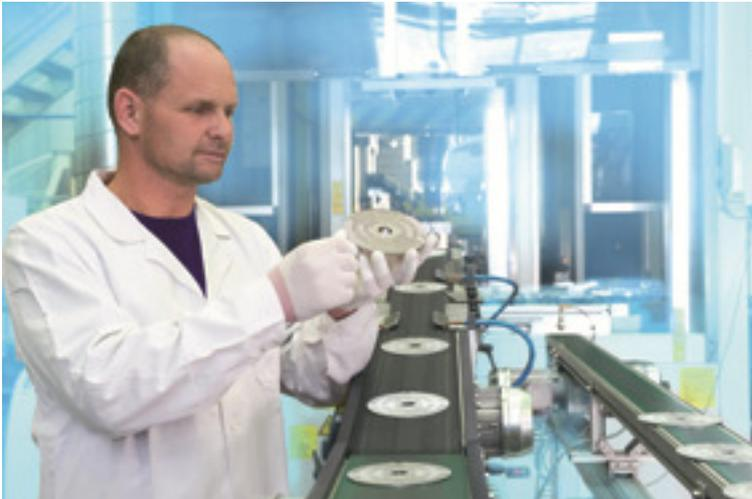
*PLANSEE produces the interconnects using a powder metallurgy net shape process.*
