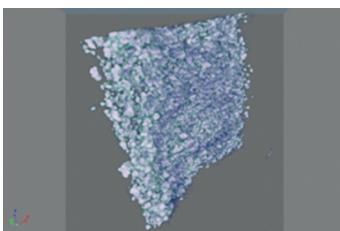
3D images provided by nano-CT scanning enables NEXT ENERGY scientists to analyse the structure of an electrode's coating.
